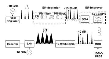
Fig. 4. Schematic of experimental setup.
