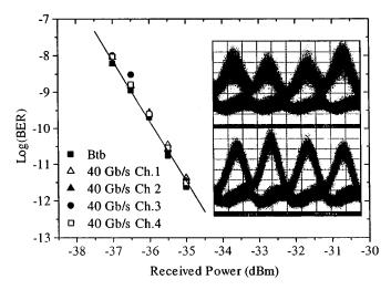
Fig. 5. BER performance of the four demultiplexed channels, compared to 10 Gb/s back-to-back. Insets: 40-Gb/s eye diagram without (upper), and with (lower) the aid of the "ER-improver."
